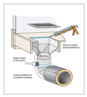
**Duct Sealing Locations at Branch and Boot**
