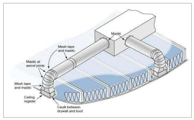
**Duct Sealing Locations at Trunk and Branches**
